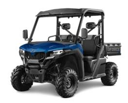
■ 580cc engine ■ 12 inch steel wheels ■ 250kg tray capacity ■ 680kg tow capacity
